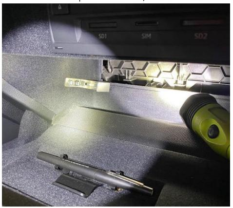
**Step 26**Mount gauge in bracket and connect harness.
