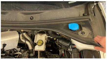
**Step 5**Remove the windshield washer reservoir cap.
